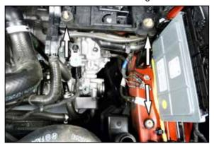
9. Install the three rubber mounted studs in the places shown.
