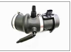
13. Install the factory mass air sensor into the K&N hose as shown but don't tighten the clamp.
