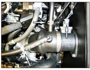
15. Reconnect the vent lines and secure with the factory spring clamps. Reconnect the mass air sensor electrical connection.
