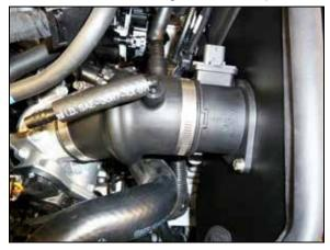
14. Install the hose/maf housing assembly onto the throttle body and into the heat shield. Adjust the maf housing so the holes line up and secure with the provided hardware. Adjust the hose for best fit and then secure with the provided hose clamps.
